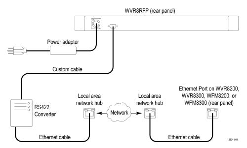
Figure 1: Ethernet connection using LAN
