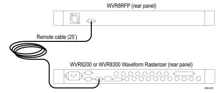
The Waveform Rasterizer provides power to the WVR8RFP through the remote cable.
