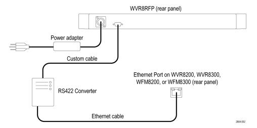
Figure 2: Ethernet connection directly to instrument
